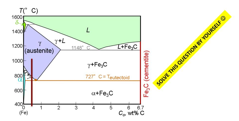
Q4. For an iron-carbon alloy of composition 5 wt% C-95 wt% Fe, make schematic sketches of the microstructure that would be observed for conditions of very slow cooling at the following temperatures: 1180°C (1453 K), 1145C, and 700°C (973 K). Label the phases and
